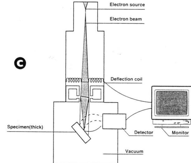
Scanning electron microscope (SEM)
